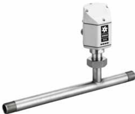
OS 420: Shortened inlet section! Recommended inlet section length is: l = 15 \times \text{inner pipe diameter}
