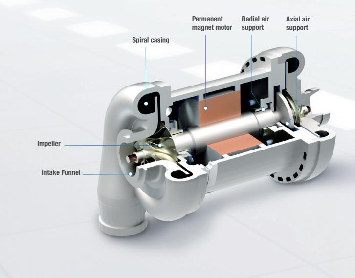
When there is no oil, then none can escape. Our new High Speed Turbo Compressors are designed so that the entire drive mechanism operates without any lubricants at all; giving you total confidence that your compressed air is 100% oil-free. A permanent magnet motor and the unique air-supported motor shaft ensure dependable low-maintenance operation with minimal energy use.
