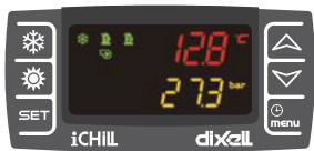
IC208CX microprocessor controller.
